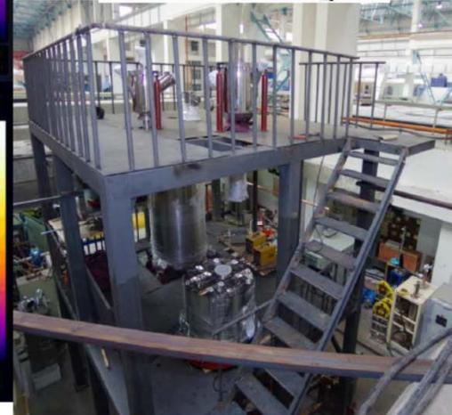
Large scale loop & HT test      Granular target test bench
