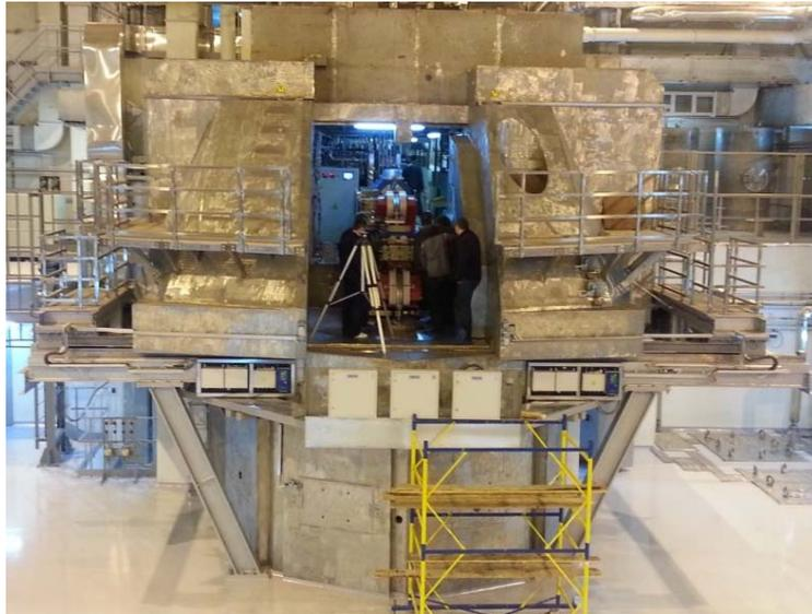
**Top shield and bending magnet**
